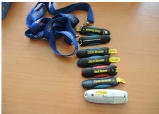
Flash Disk Corsair 2GB USB 2.0; USB Flash Voyager - 1 GB/2GB; OPE1467, OPE1468, OPE1488, OPE1509
